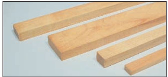
Used to take-up space and provide stable lock-up for quoin. Available in 36" lengths, 5/8" tall, in a variety of picas.
