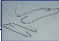
Mounted and unmounted printing plates hang on special "S" hooks, which are available in two sizes:
