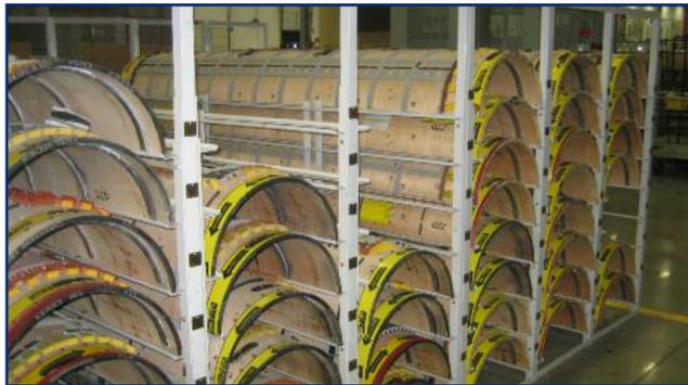
Wagner can supply specialized Henderson Storage Systems for just about any type of die, including **DRO and EVOL rotary dies**. These heavy-duty units are designed to be sturdy, durable and versatile. Transfer carts are also available. All DRO and EVOL racks and carts come in white powder-coated finish.
