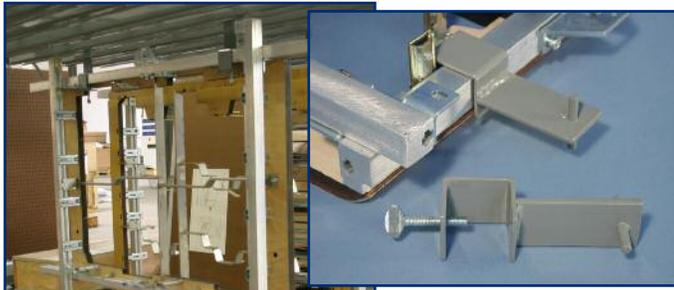
**Easi Blank Hangers** - from Wagner allow easy and secure storage of blankers along with corresponding Bobst dies. These brackets are easy to use, and can be adjusted for a secure hold by a thumbscrew. Easi Hangers are available in pairs and are designed to fit Henderson Storage Racks using 5-1/2" Bobst sections. Contact Wagner for more details!
