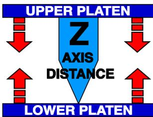
between the upper steel rule die and the lower cutting plate. This is referred to as setting the “Z-Axis Gap.” **See left.** The third problem is making sure pressure is balanced from one side of the press to the other. In other words the gap is identical on both sides, and in fact on all sides of the press, so the application of pressure is evenly balanced
